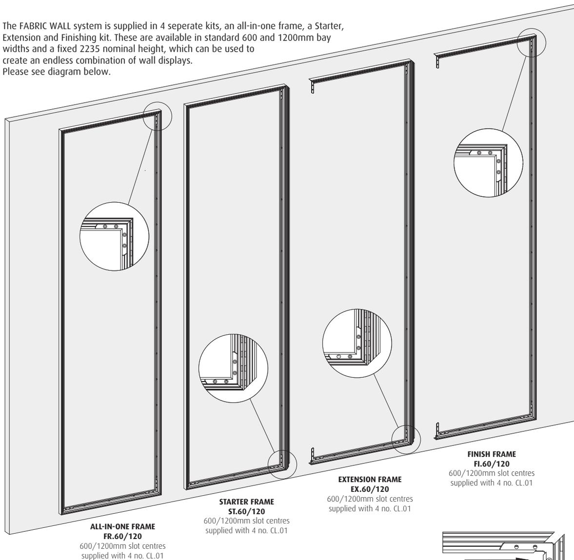
All 4 kit variations are supplied with 4 no. CL.01 fixing 'L' brackets. For ease of construction, all profiles are mitred at 45 degrees both ends. Simply slide the two profiles flush then fix in place with 4 screws supplied.
